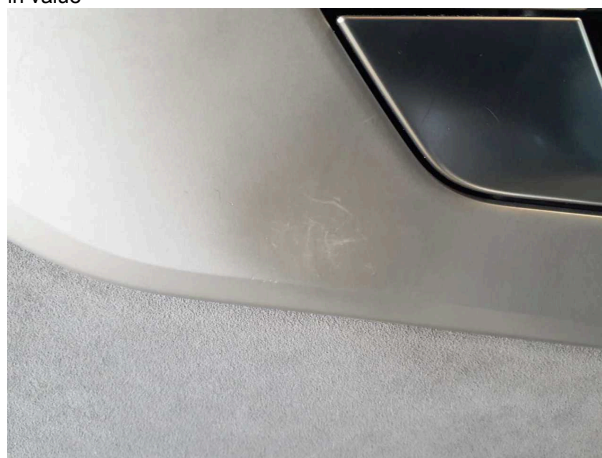
Damage #4: Trim / covers: Brightware / decorative strip (türverkleidung VL) - Scratched - Replace
