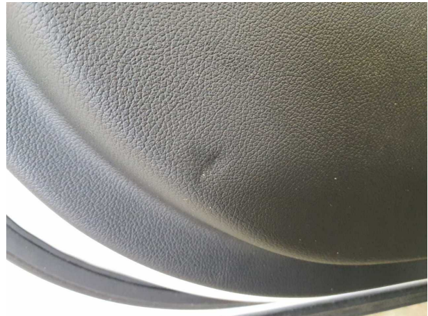
Damage #1: Trim / covers: Door trim - front left side - Deform... - Loss in value
