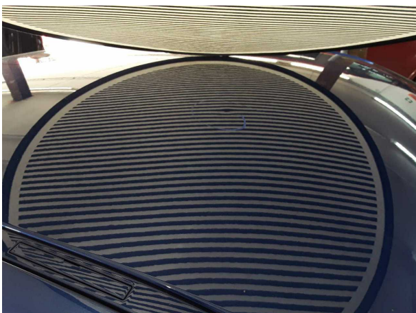
Damage #3: Roof: Roof - dent(s) - Smooth repair work
