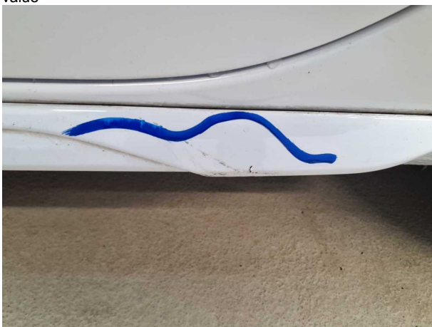
Damage #6: Sill - left side: Trim - Scratched - Smart repair
