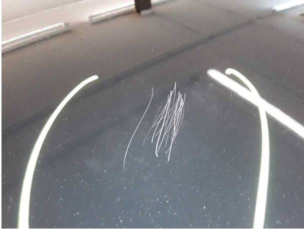
Damage #5: Roof: Roof - Scratched - Repair and paint
