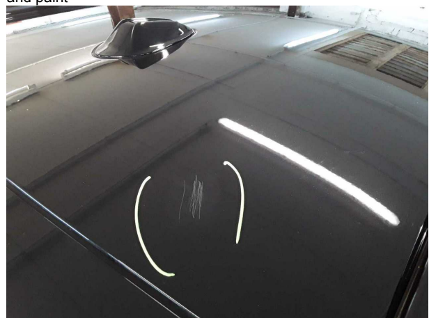
Damage #5: Roof: Roof - Scratched - Repair and paint
