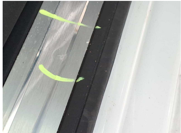
Damage #1: Trim / covers: Brightware / decorative strip (Vr Einstiegsleiste) - dent(s) - Replace
