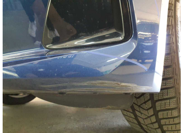
Damage #6: Front bumper: Front bumper - Scratched - Repair and paint
