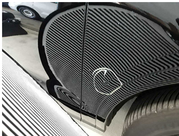
Damage #4: Mudguard - right side: Mudguard - right side - dent(s) - Smooth repair work
