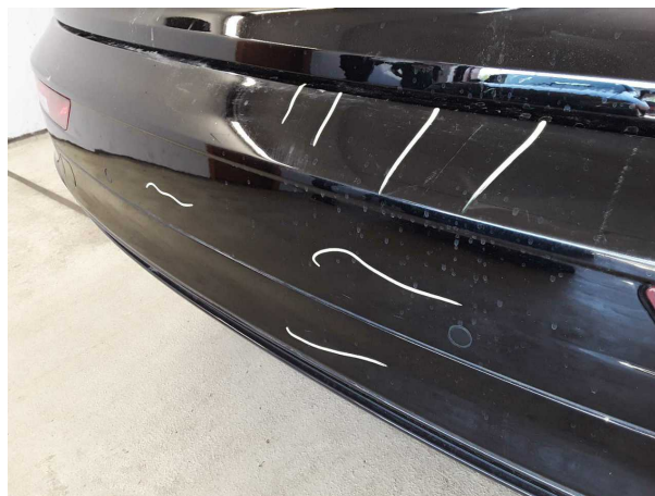
Damage #7: Rear bumper: Rear bumper - Scratched - Paint
