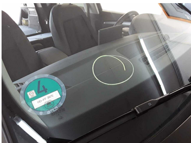
Damage #8: Vehicle glazing: Windscreen - Stone chips - Replace
