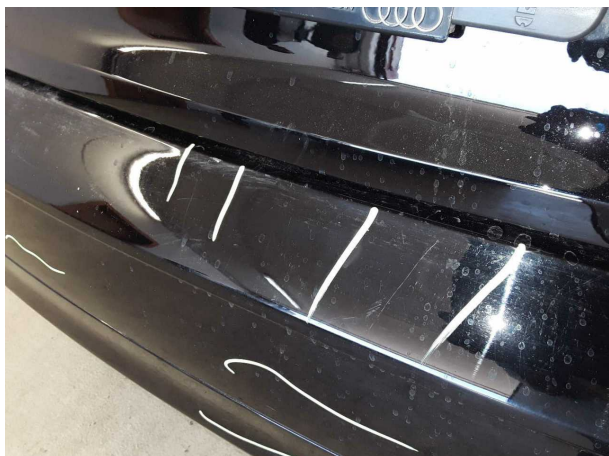
Damage #7: Rear bumper: Rear bumper - Scratched - Paint
