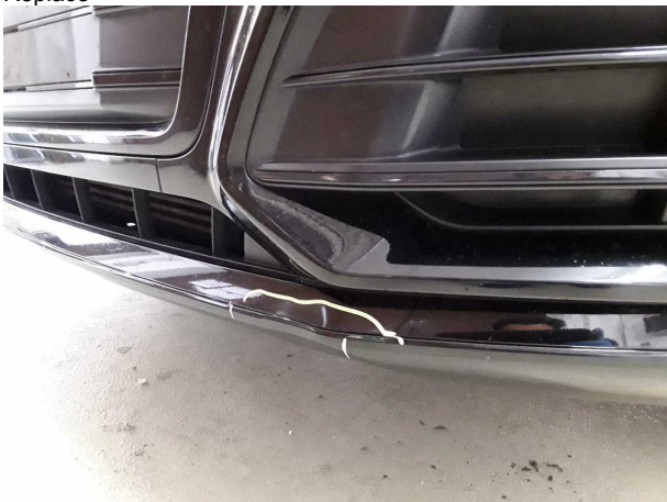
Damage #9: Front bumper: Front bumper (Verformt) - Scratched - Replace
