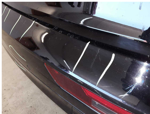
Damage #7: Rear bumper: Rear bumper - Scratched - Paint
