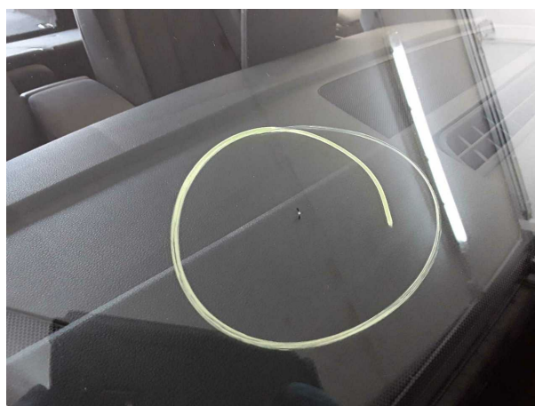
Damage #8: Vehicle glazing: Windscreen - Stone chips - Replace
