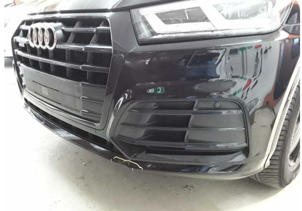
Damage #9: Front bumper: Front bumper (Verformt) - Scratched - Replace
