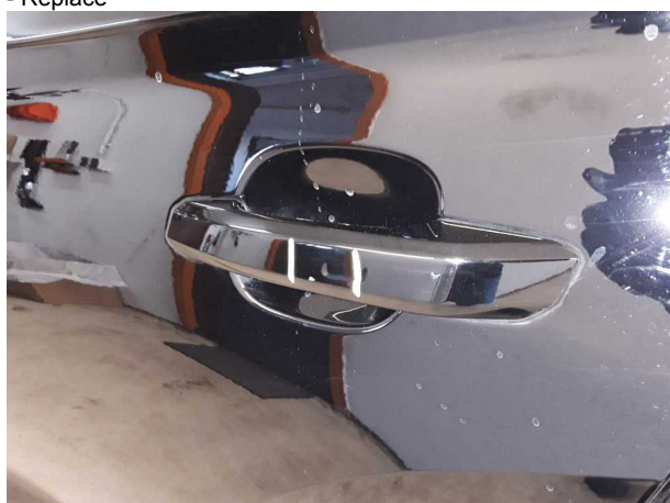
Damage #3: Door - rear left side: Door handle - outside - Scratched - Smart repair
