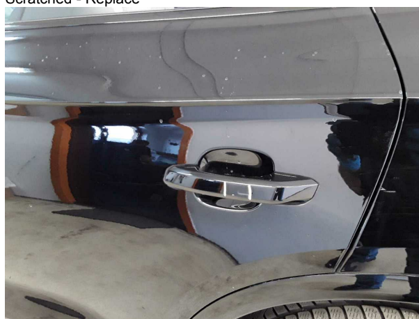
Damage #3: Door - rear left side: Door handle - outside - Scratched - Smart repair
