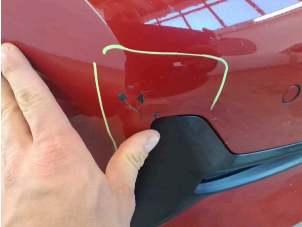
Damage #4: Front bumper: Front bumper (Gebrochen) - Damaged - Replace
