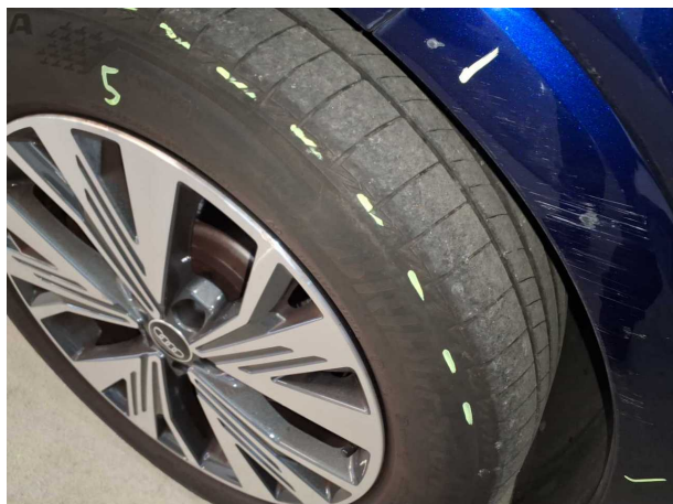
Damage #7: Wheel / tyres: Tyre - front - Expired - Replace
