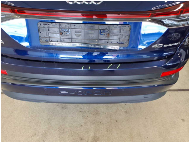
Damage #2: Rear bumper: Rear bumper - Scratched - Cover / polish
