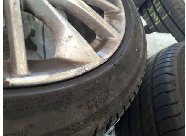
Damage #10: 2nd wheel set: 1 alloy rim - Scratched - Replace
