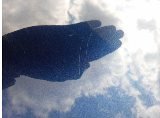
Damage #4: Roof: Roof - Scratch(es) - Smart repair
