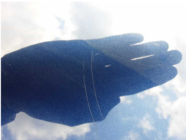
Damage #4: Roof: Roof - Scratch(es) - Smart repair
