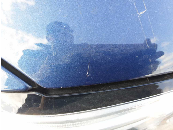
Damage #6: Bonnet: Bonnet - Scratch(es) - Smart repair
