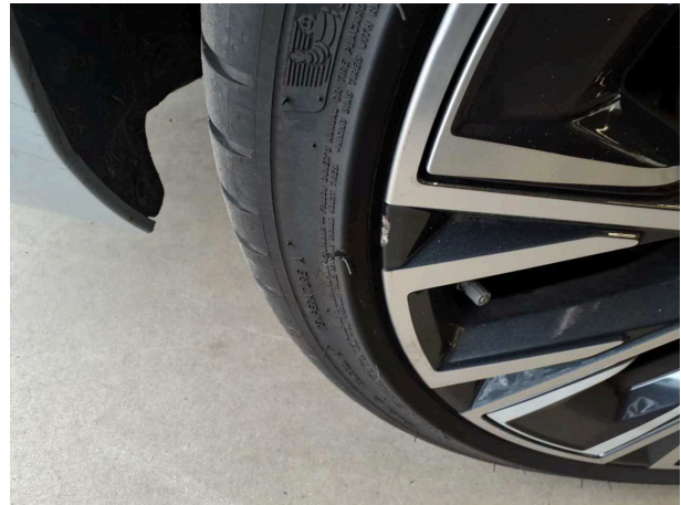
Damage #2: Wheel / tyres: Tyre - rear right side - Damaged - Replace
