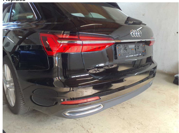
Damage #6: Rear bumper: Rear bumper - Scratched - Paint
