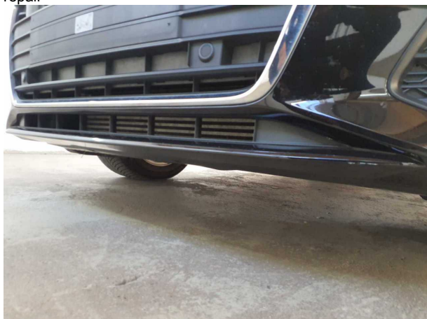
Damage #2: Front bumper: Spoiler - Scratched - Smart repair
