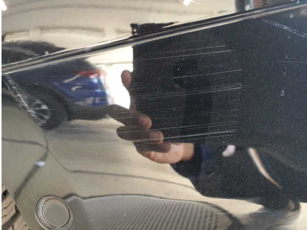
Damage #6: Rear bumper: Rear bumper - Scratched - Paint
