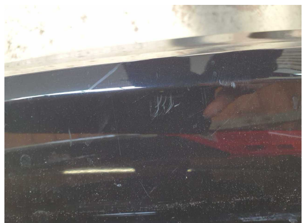
Damage #6: Rear bumper: Rear bumper - Scratched - Paint
