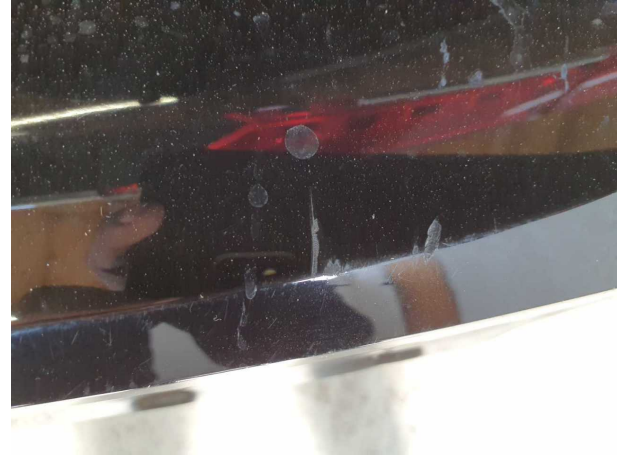
Damage #6: Rear bumper: Rear bumper - Scratched - Paint
