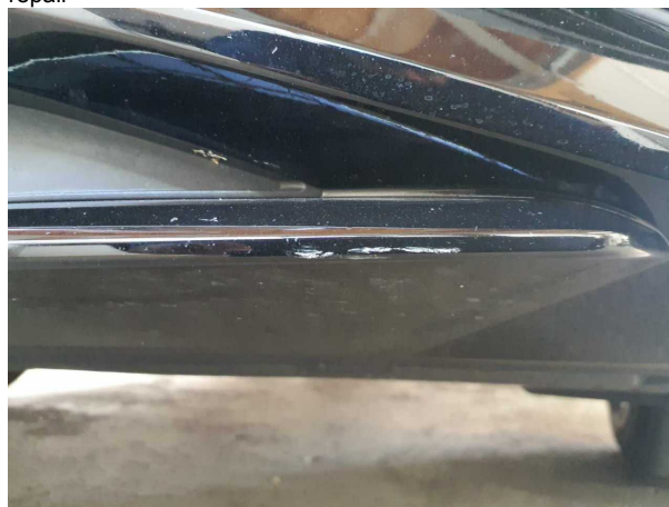
Damage #2: Front bumper: Spoiler - Scratched - Smart repair
