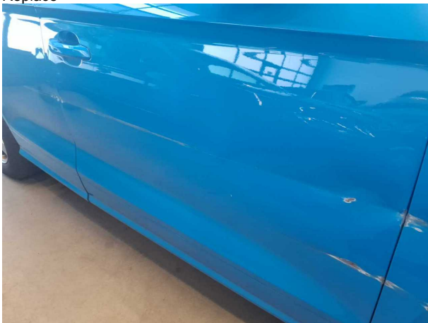
Damage #14: Door - front right side: Door - Scratched - Replace
