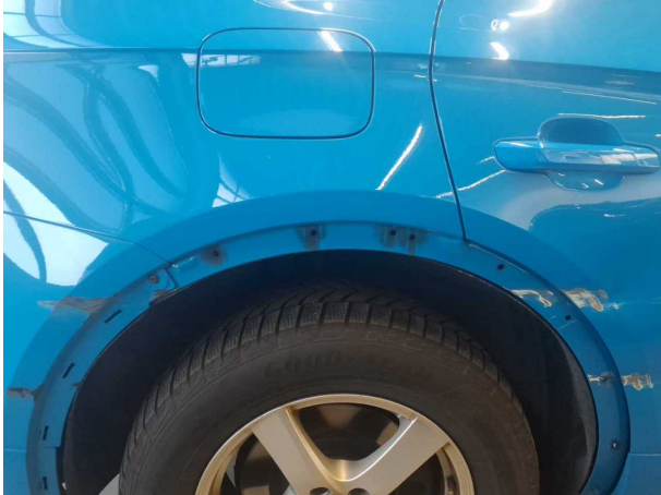
Damage #6: Side panel - rear right side: Wheel well extension - Missing - Replace
