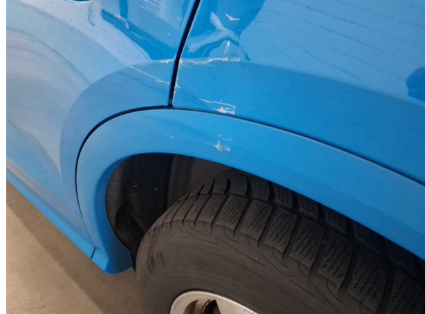
Damage #2: Side panel - rear left side: Wheel well extension - Scratched - Repair and paint
