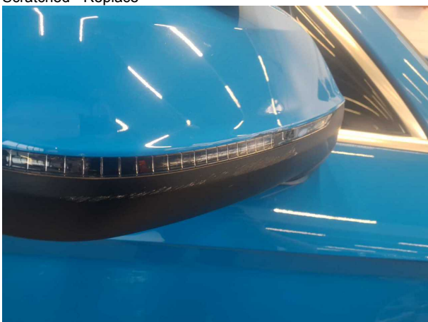
Damage #5: Wing mirror - right side: Cap - Abrasion - Replace
