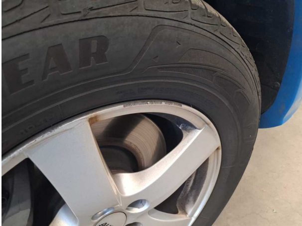
Damage #12: Wheel / tyres: Alloy rim - front right side - Damaged - Replace
