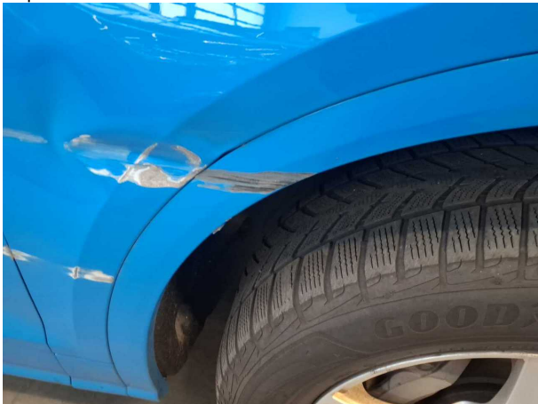
Damage #4: Mudguard - right side: Wheel well extension - Scratched - Replace
