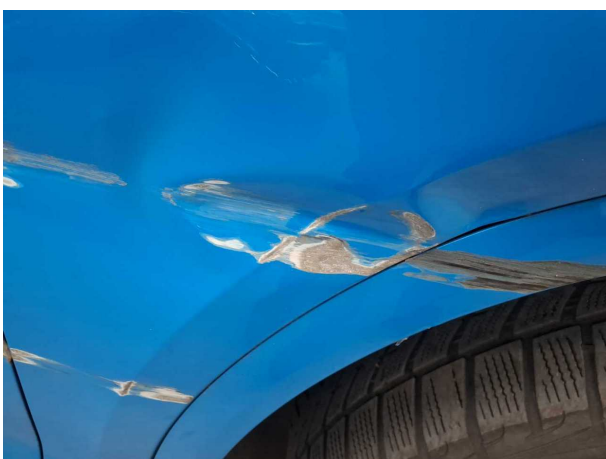
Damage #10: Mudguard - right side: Mudguard - right side - Scratched - Replace
