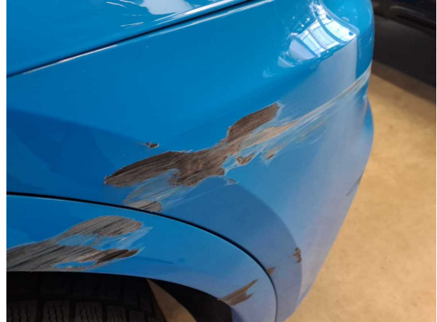
Damage #13: Front bumper: Front bumper - Scratched - Replace
