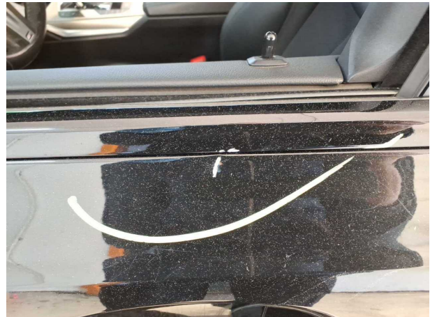
Damage #2: Door - front left side: Brightware - upper - Damaged - Replace
