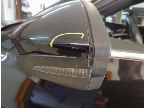
Damage #3: Wing mirror - left side: Cap - Scratched - Paint
