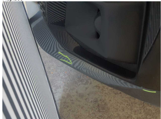
Damage #11: Front bumper: Front bumper - Deformed - Replace
