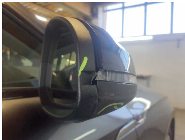
Damage #4: Wing mirror - right side: Mirror housing - Damag... - Replace
