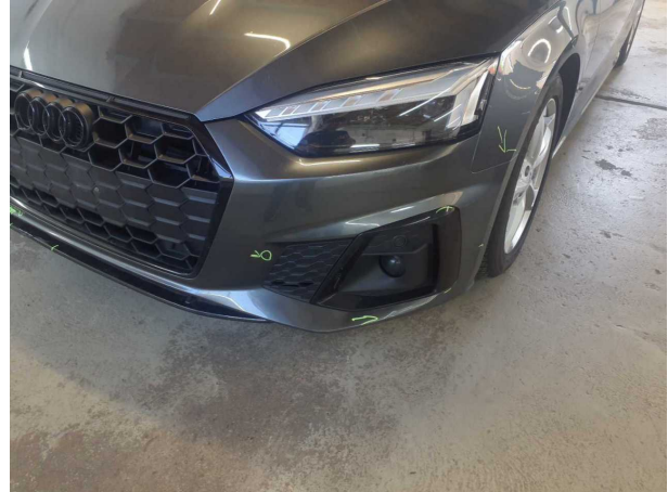
Damage #11: Front bumper: Front bumper - Deformed - Replace
