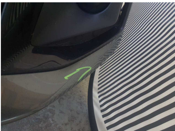
Damage #11: Front bumper: Front bumper - Deformed - Replace
