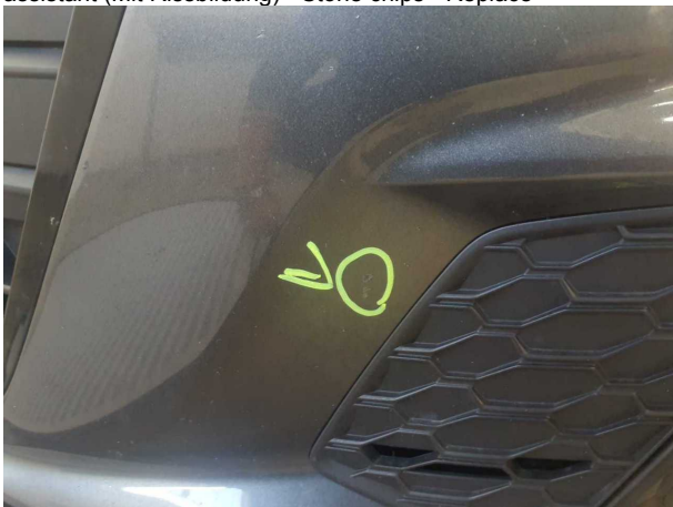
Damage #11: Front bumper: Front bumper - Deformed - Replace
