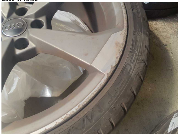
Damage #6: 2nd wheel set: Alloy rim set - complete - Scratched - Loss in value
