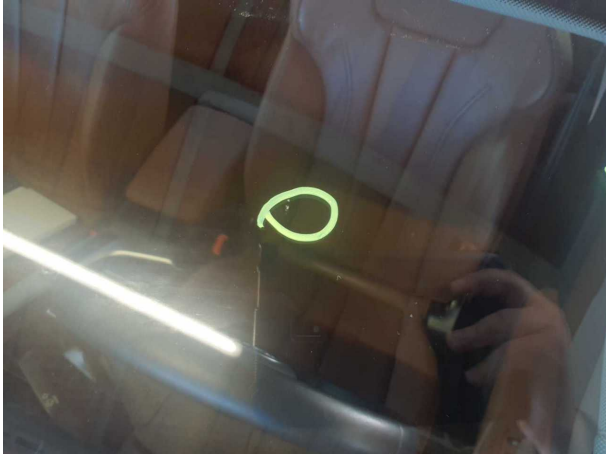
Damage #10: Vehicle glazing: Windscreen with lane departure assistant (Mit Rissbildung) - Stone chips - Replace
