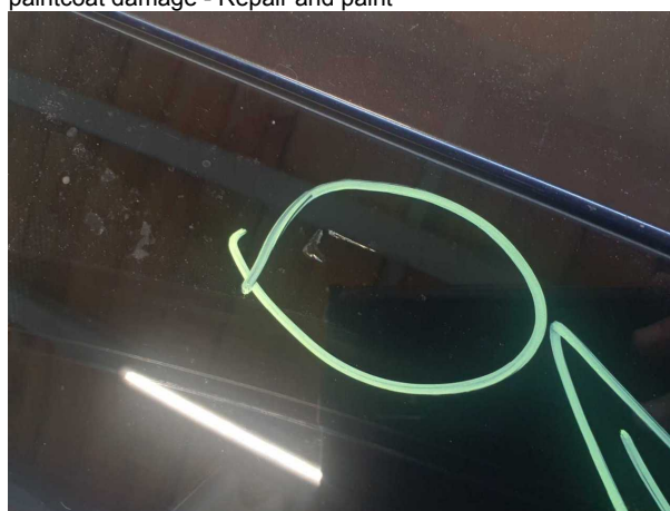
Damage #10: Vehicle glazing: Windscreen with lane departure assistant (Mit Rissbildung) - Stone chips - Replace
