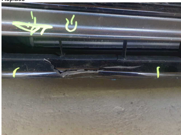
Damage #5: Front bumper: Spoiler - Damaged - Replace
