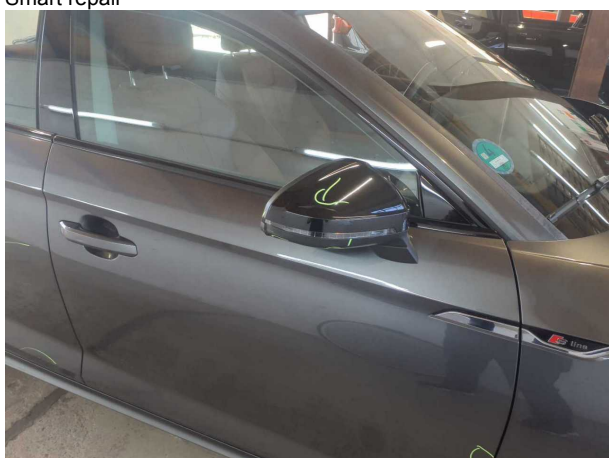
Damage #4: Wing mirror - right side: Mirror housing - Damaged - Replace
