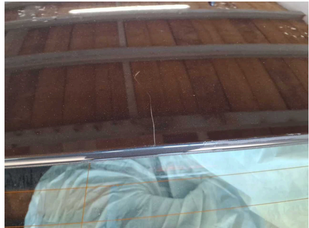
Damage #2: Boot lid / rear door: Rear spoiler - Scratch(es) - Paint
