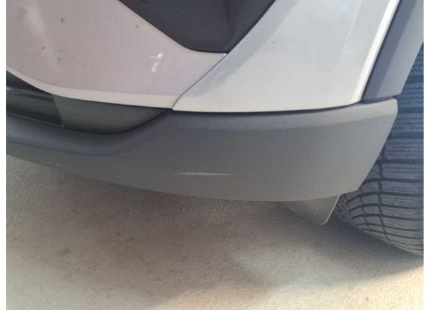
Damage #5: Front bumper: Spoiler - Scratch(es) - Loss in value
