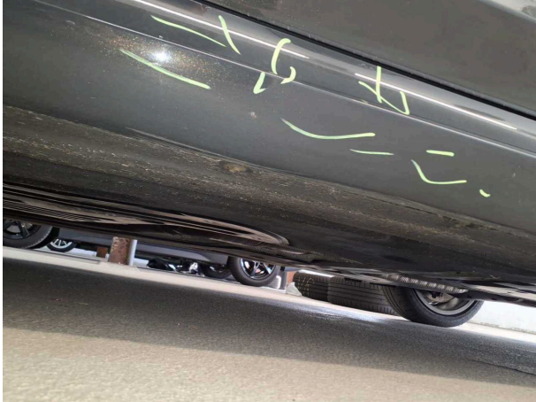
Damage #9: Sill - left side: Trim - Scratched - Smart repair
