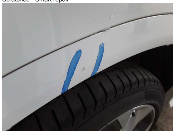
Damage #6: Side panel - rear right side: Wheel well extension - Scratched - Smart repair
