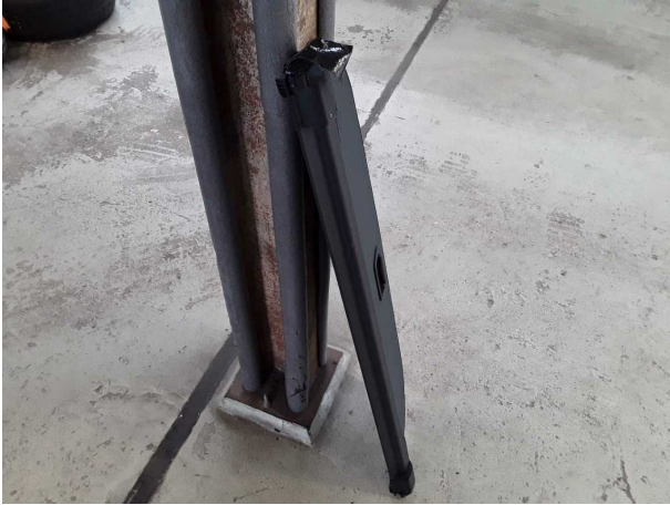
Damage #7: Interior: Boot cover / roller cover - Broken / torn - Replace
