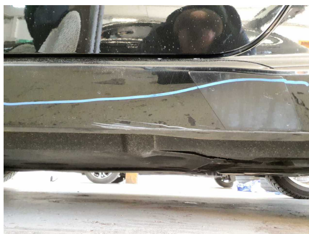
Damage #7: Sill - left side: Trim - Scratched - Replace
