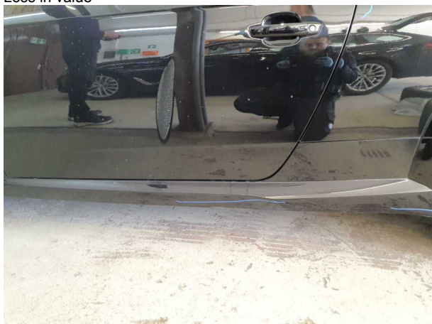
Damage #7: Sill - left side: Trim - Scratched - Replace
