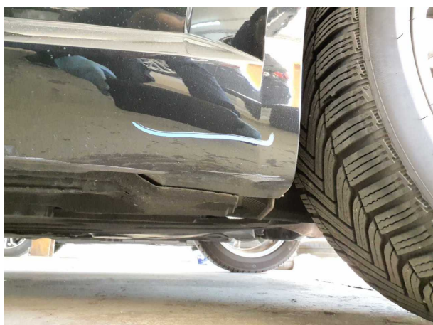
Damage #7: Sill - left side: Trim - Scratched - Replace
