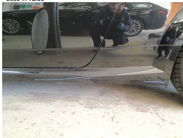
Damage #7: Sill - left side: Trim - Scratched - Replace
