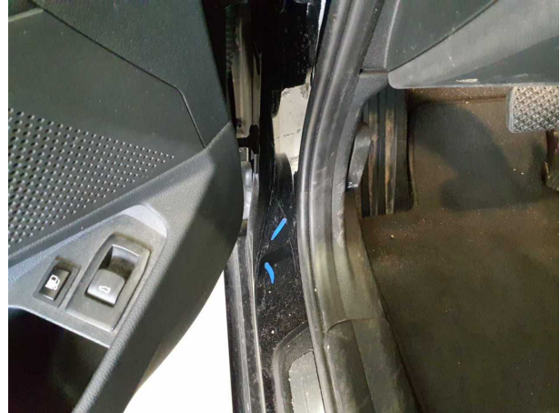
Damage #7: Sill - left side: Sill - Scratch(es) - Smart repair
