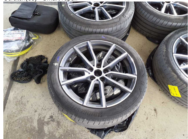
Damage #12: 2nd wheel set: 2 alloy rims - Scratched - Loss in value
