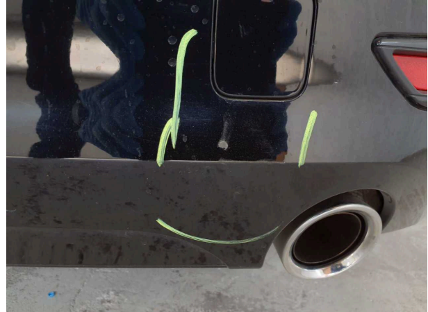
Damage #18: Rear bumper: Rear bumper - Damaged - Replace
