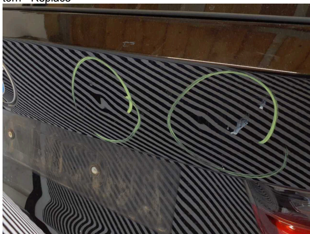
Damage #15: Boot lid / rear door: Boot lid - Dent / paintcoat damage - Repair and paint
