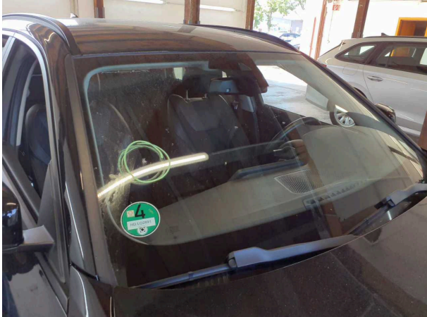
Damage #9: Vehicle glazing: Windscreen - Stone chips - Replace
