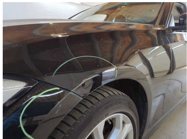
Damage #8: Mudguard - left side: Mudguard - left side - Dent / paintcoat damage - Repair and paint
