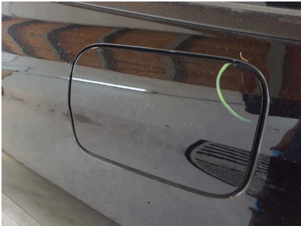
Damage #1: Fuel system: Tank cap - Scratched - Smart repair
