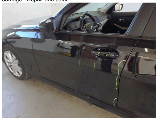
Damage #16: Door - front left side: Door - Scratched - Repair and paint
