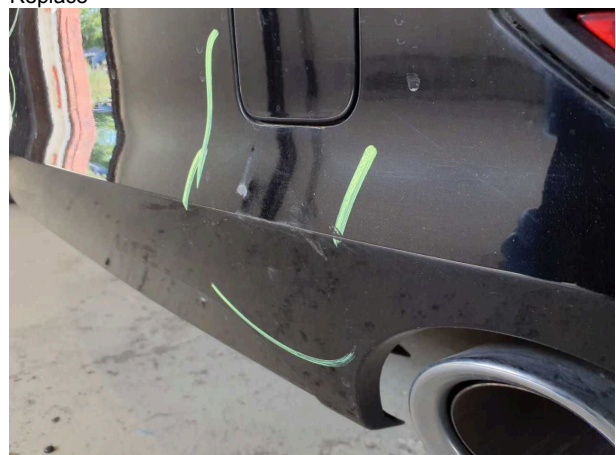
Damage #18: Rear bumper: Rear bumper - Damaged - Replace
