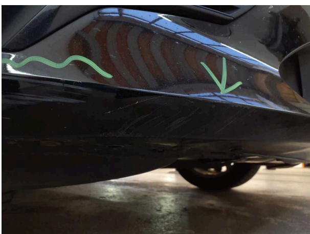
Damage #19: Front bumper: Front bumper - Damaged - Replace
