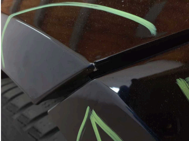
Damage #11: Mudguard - right side: Mudguard - right side - Broken / torn - Replace
