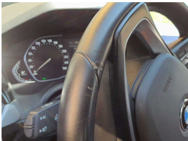
Damage #14: Steering system: Steering wheel sheath - Broken / torn - Replace
