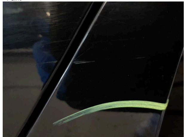
Damage #12: Side panel - rear left side: Side panel - Scratch... - Paint
