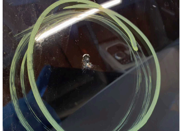
Damage #9: Vehicle glazing: Windscreen - Stone chips - Replace
