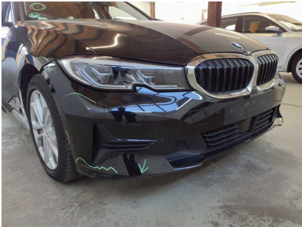
Damage #19: Front bumper: Front bumper - Damaged - Replace
