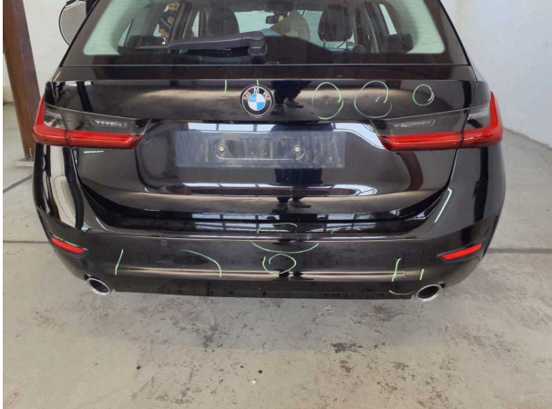
Damage #18: Rear bumper: Rear bumper - Damaged - Replace
