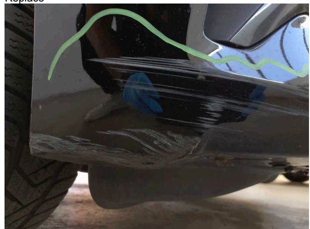
Damage #19: Front bumper: Front bumper - Damaged - Replace
