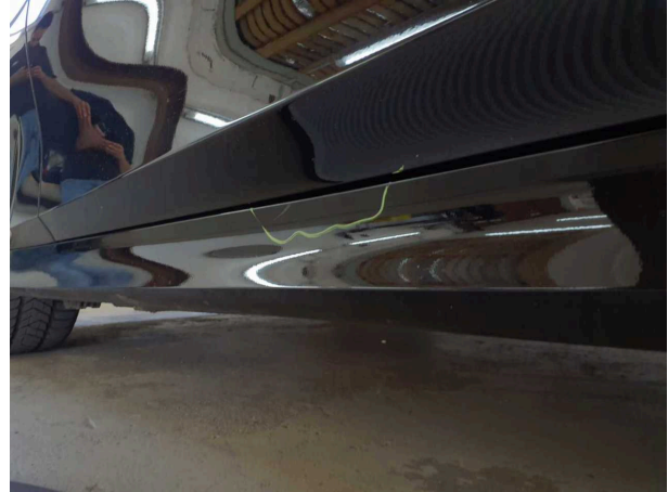
Damage #7: Sill - left side: Trim - Scratched - Paint
