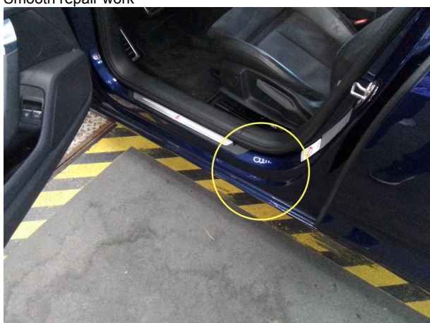
Damage #3: Sill - left side: Sill - Scratched - Smart repair
