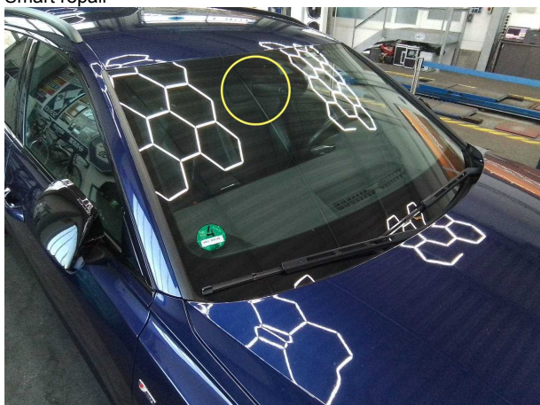
Damage #6: Vehicle glazing: Windscreen (Steinschlag) - Broken / torn - Replace
