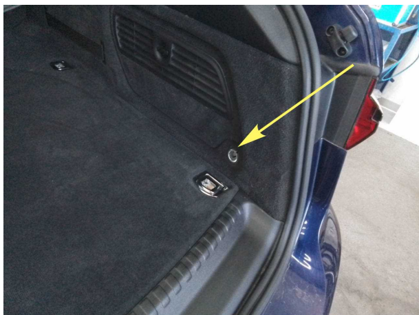
Damage #1: Trim / covers: Boot lining (Abdeckung 12 Volt) - Missing - Replace
