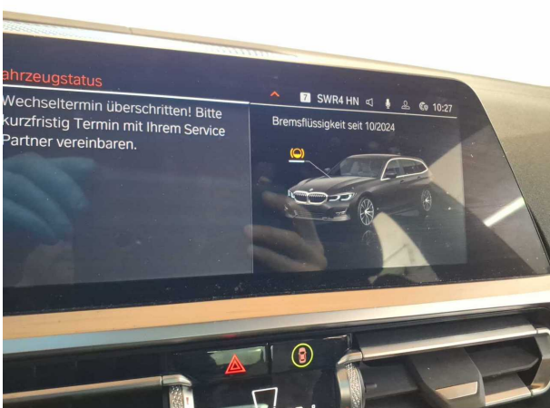
Damage #2: Braking system: Brake fluid - Due - Replace
