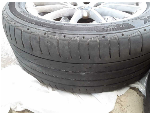
Damage #4: 2nd wheel set: 2 tyres - Worn - Replace
