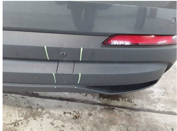
Damage #6: Rear bumper: Spoiler - Damaged - Replace
