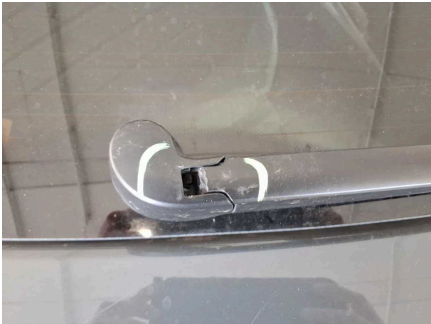
Damage #2: Screen cleaning: Wiper arm - rear - Damaged - Replace
