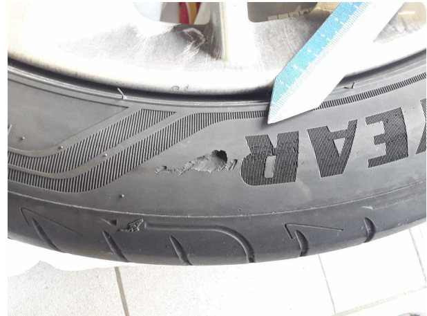
Damage #1: 2nd wheel set: 1 tyre - Damaged - Replace
