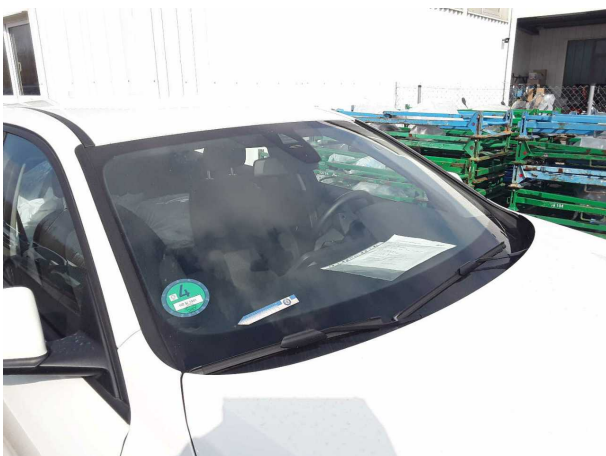
Damage #4: Vehicle glazing: Windscreen - Stone chips - Replace
