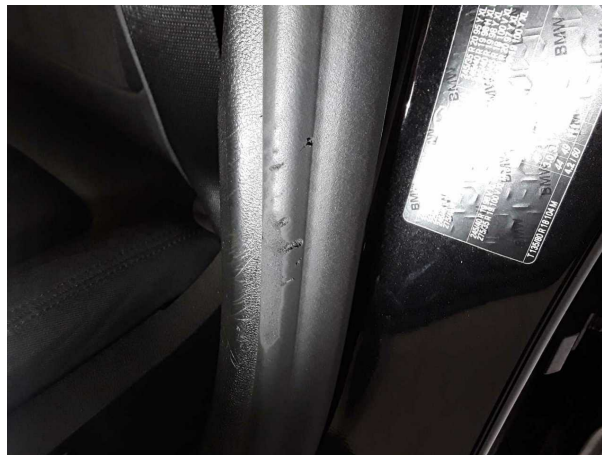
Damage #10: Body: Door seal - front left side - Damaged - Replace
