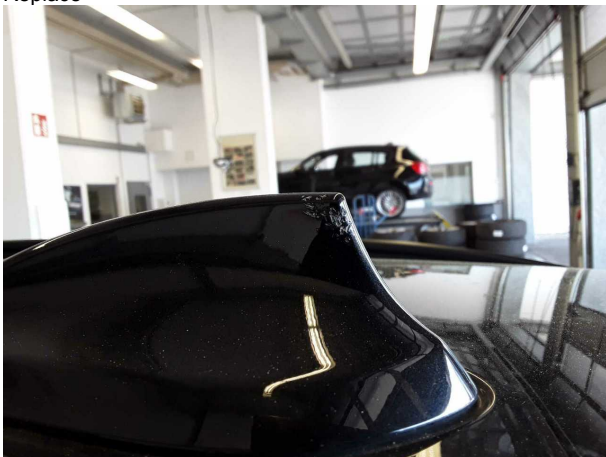
Damage #13: Roof: Aerial - Damage caused by marten / rodent - Replace
