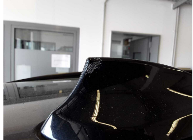
Damage #13: Roof: Aerial - Damage caused by marten / rode... - Replace
