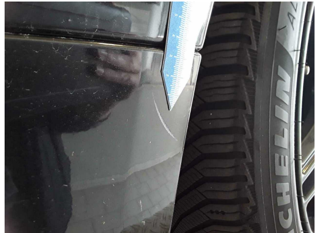
Damage #1: Sill - left side: Trim - Scratched - Smart repair
