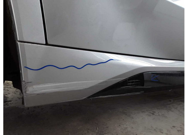
Damage #4: Sill - right side: Trim - Scratched - Replace
