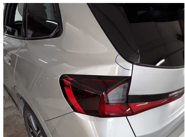
Damage #6: Side panel - rear left side: Side panel - Scratched - Paint
