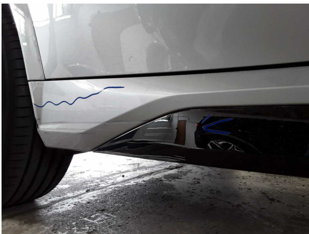
Damage #4: Sill - right side: Trim - Scratched - Replace
