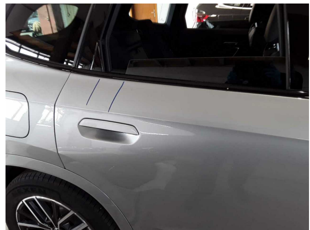
Damage #5: Door - rear right side: Door - Scratched - Paint
