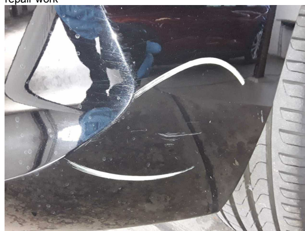
Damage #3: Rear bumper: Rear bumper - Scratched - Smart repair work
