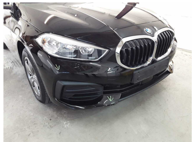
Damage #6: Front bumper: Front bumper - Deformed - Replace
