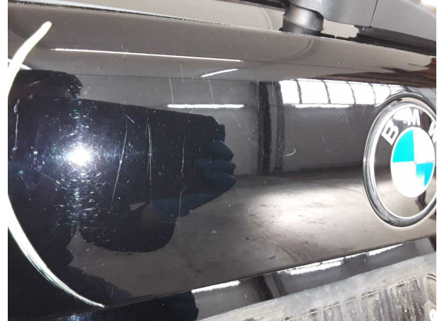
Damage #4: Boot lid / rear door: Boot lid - Scratched - Paint
