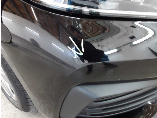
Damage #6: Front bumper: Front bumper - Deformed - Replace
