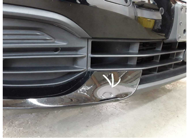
Damage #6: Front bumper: Front bumper - Deformed - Replace
